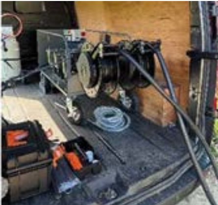
The van-based filtration setup allows technicians to carry out in-situ fuel polishing and contamination removal without requiring fuel tank removal or on-site processing.
