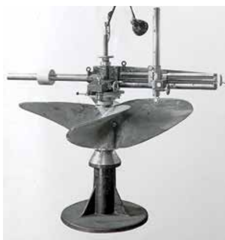
Propellermeßgerät an aeroplane propeller measuring device designed and manufactured by Haa
