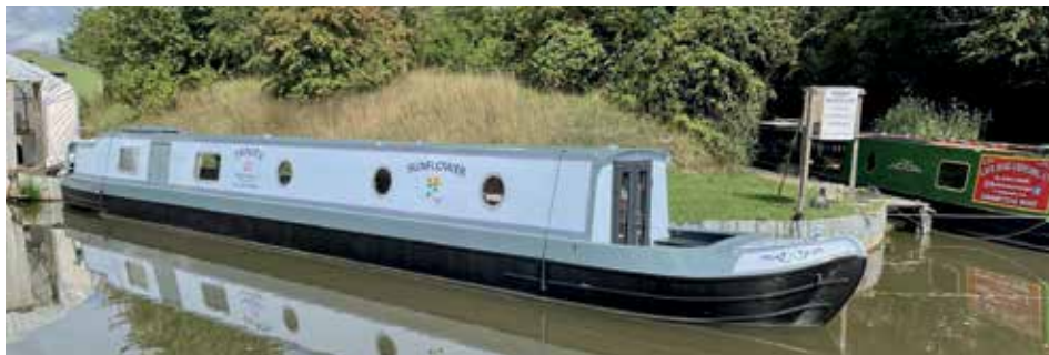
Sunflower – one of Trinity Boats' five holiday hire narrowboats and its first serial hybrid. It has a backup generator which will now run on HVO.
