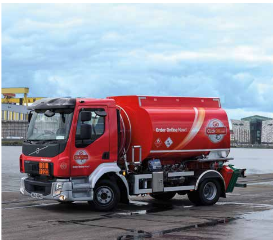
Featuring a Volvo FL 12 tonne chassis and 7,000 litre three compartment tank, this recent Morrow Tanker Services build was for the LCC Group's Go Click Oil.com brand
