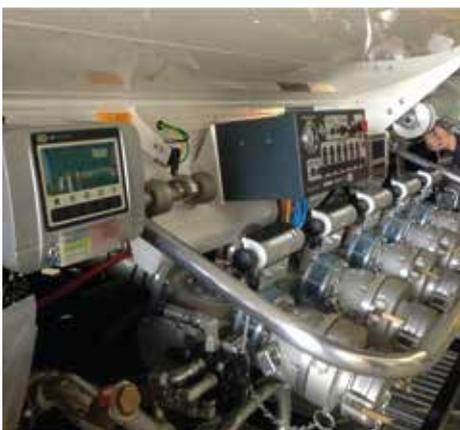
electronic data on fuel movements between bulk storage tanks and road tankers. This provides essential information for wet stock management. They also provide added levels of security including pin code access and the capture of driver and vehicle data."
