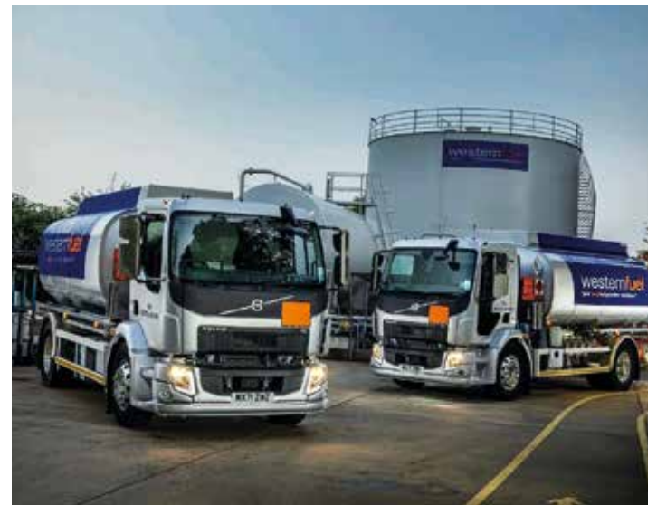
Western Fuels’ new build with 13000ltr, 4 compartment, ring tank with Emco Wheaton BLVR system.
