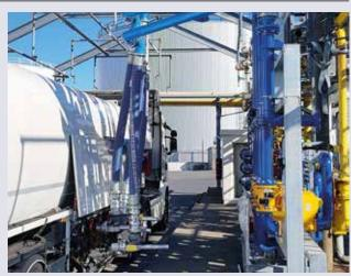
Carbis Loadtec LA210 bottom hose loading skid
