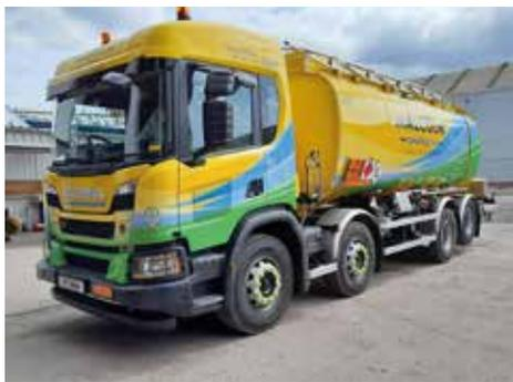
"Fuel is our speciality so an Aluminium 20,000ltr single compartment barrel was fitted to the front of the chassis along with an Alpeco metering system with product return and bulk delivery.
