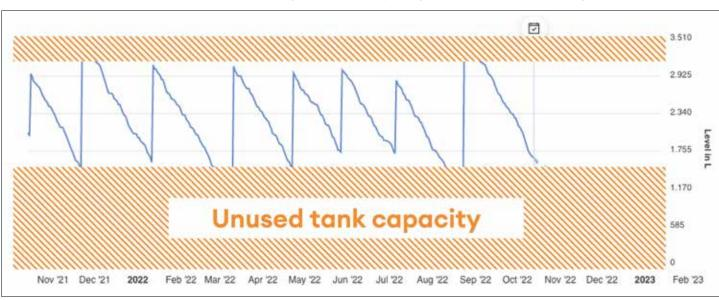
Figure 1: A fill level history with consumption and delivery patterns as it is shown in the FoxPortal, FoxInsights' central platform that provides a detailed overview of all customers' tanks fill levels. In this example, the tank capacity used is only about 42%, resulting in short refill intervals. This means that deliveries are made far too early and thus money is lost
