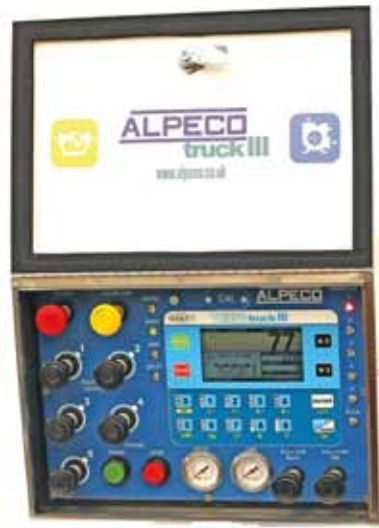
Equipped with real-time inventory software, Alpeco's Truck III allows the operator to enter grade and product volume into each compartment
