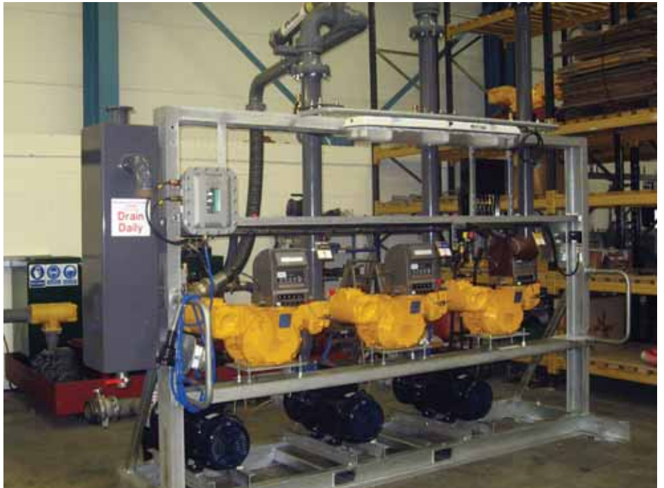
Kerosene is pumped through each flow line at a rate of up to 1100 litres per minute using IFC Inflow's purpose-built skid testing facility to ensure that new skids will run smoothly and without problems from day one
