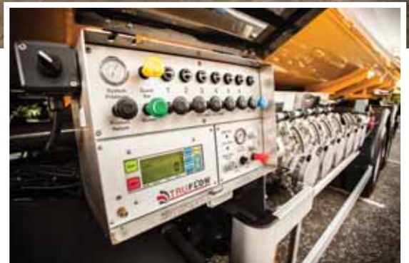
Now operating in Malta, this tanker features a TruFlow 1000 electronic bulk meter system designed by the Maine Group
