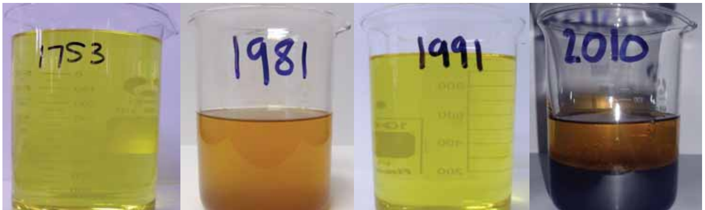
A fuel line up – these samples show the variable quality of fuel which ranges from clean kerosene with a char value of 6.5mg/kg taken from a distributor's tank to dirty kerosene, clean kerosene but with a high (off spec) char value to really dirty kerosene
