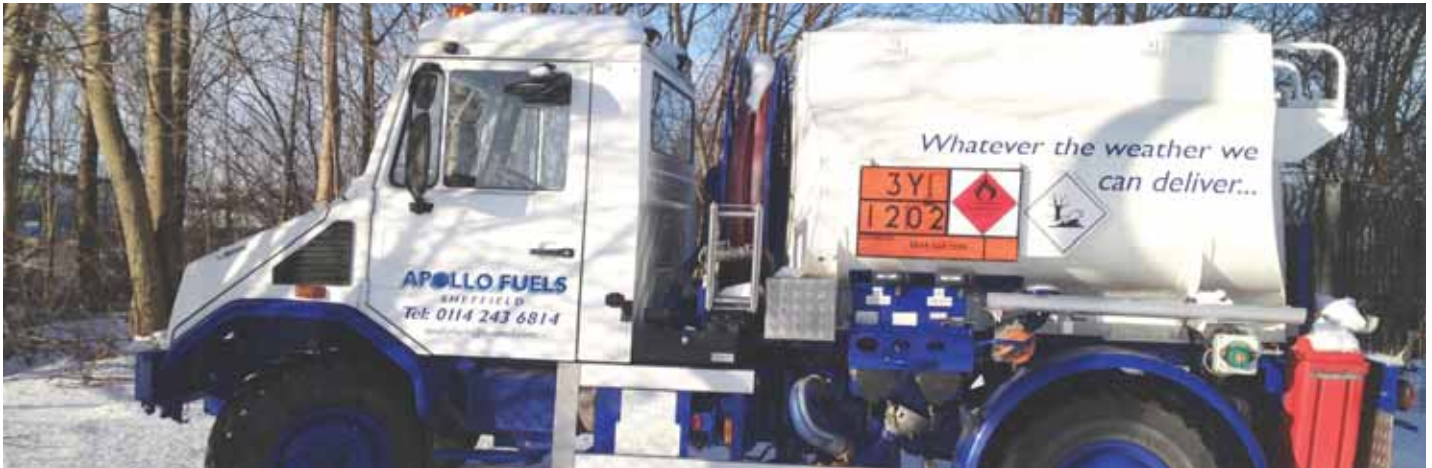
Helping out Apollo Fuels customers in the snowy weather is this 4x4 Mercedes all terrain tanker. Built by Road Tankers Northern, the vehicle features a two compartment 2500 litre aluminium tank with Gardner Denver Drum bottom loading manifold and electronic meter system
