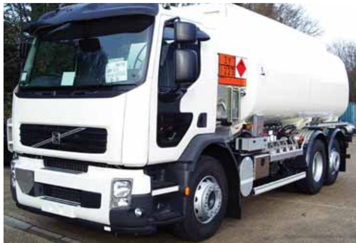
The standard specification of a Haartz rigid is a six-wheel, four-compartment tanker with rear steer. This Volvo joined the Haartz fleet in November
