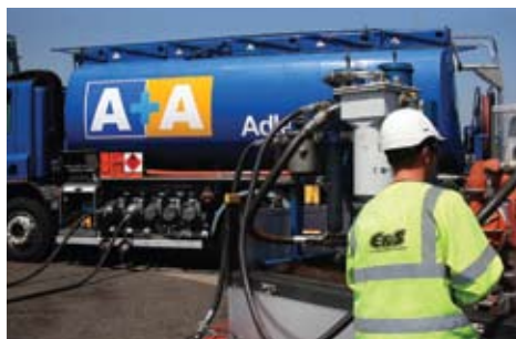
On site fuel polishing with Adler and Allan
